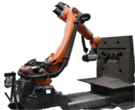
Badger Alloys now offers patternless molding with this 6-axis robotic milling center.
