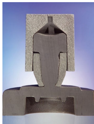
Figure 1: Cross section of Tele-Feeder
